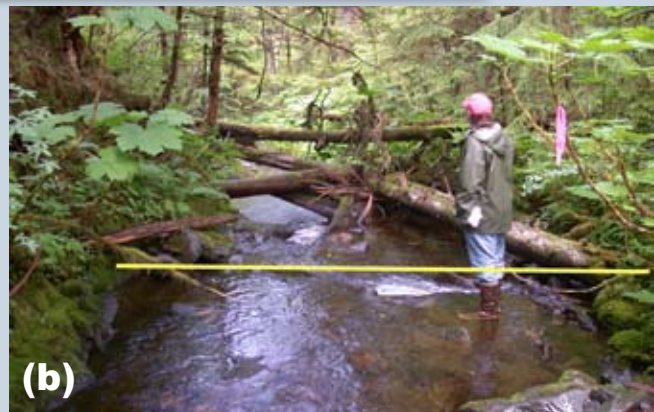
Figure 5.5—(a) Bankfull elevation on an unentrenched alluvial channel. (b) Ordinary high water elevation in an entrenched coarse-grained channel without depositional features.
